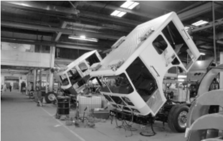
Two of the many Seagrave fire vehicles currently under construction at the Clintonville plant; cabs on most of the trucks tilt forward like this for access to the engine and other components.
