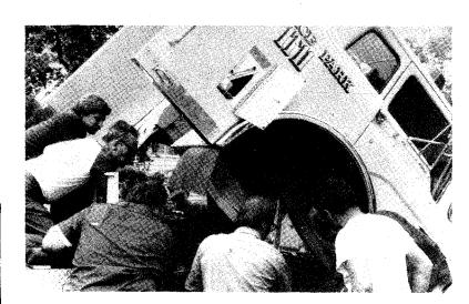
Members of the fire department tilt up the cab and study the eight-cylinder diesel engine that powers the vehicle and the pump that's conservatively rated at 1000 gallons a minute capacity.
